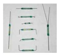
Most Contacts can be made open loop, closed loop, SPDT, DPDT at your request. All contacts are made with "standard" reeds except for SPDT and Open Loop.
