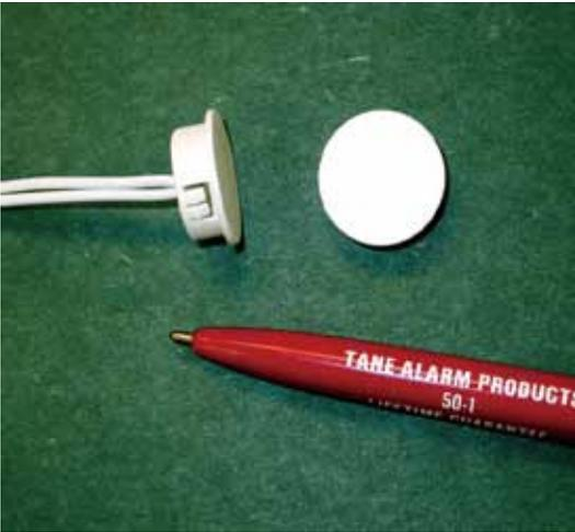
The Tane Mini-Disc is a unique contact as it has a wide gap for its slim size
