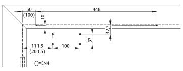
Installation dimensions for direct standard mounting non hinge side
